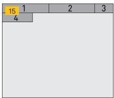
Place the Parky floor parallel to the long wall of the room. Place the floors from left to right, with the tooth side facing the beginning wall.
